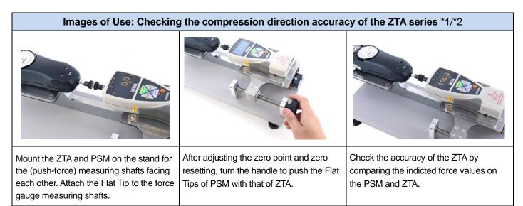
\*1 Recommended to use the same capacity range of both force gauges.
