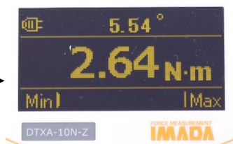
The Angle data output from the ACMTS is displayed in DTXA
