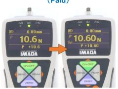
This function lowers the minimum value that can be displayed on a force gauge by one digit.
