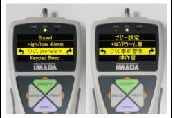
The Overload Pre-Alarm Function will sound from the time the measuring instrument reaches 90% of the maximum force value.
