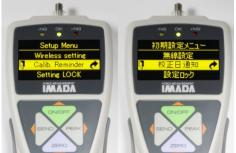
The Calibration Reminder Function displays the scheduled calibration date, from 30days before the preregistration date. You may find it useful for systematic calibration management and prevention of forgetting calibration.
